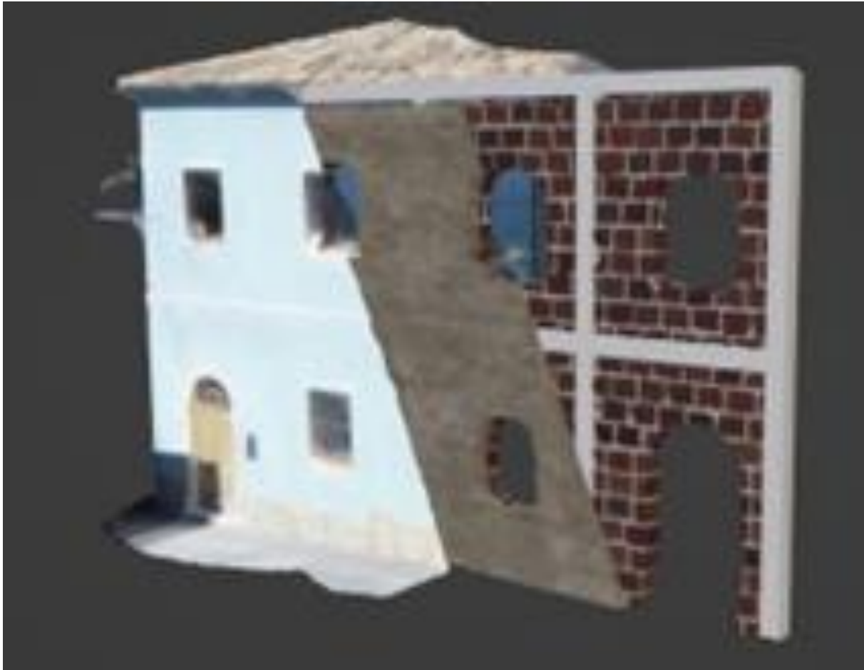
Figure 20. Wall section after the enhancement, where the external layer is derived by the 3D scan, while the other ones are added
